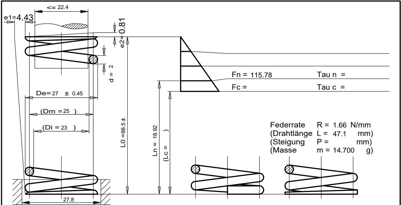
Federrate  $R = 1.66 \text{ N/mm}$
