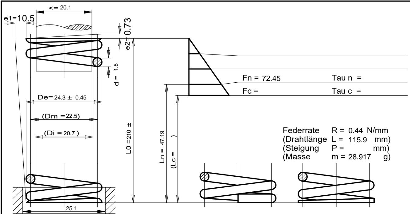
Federrate  $R = 0.44 \text{ N/mm}$
