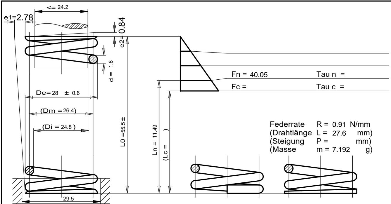
Federrate  $R = 0.91 \text{ N/mm}$
