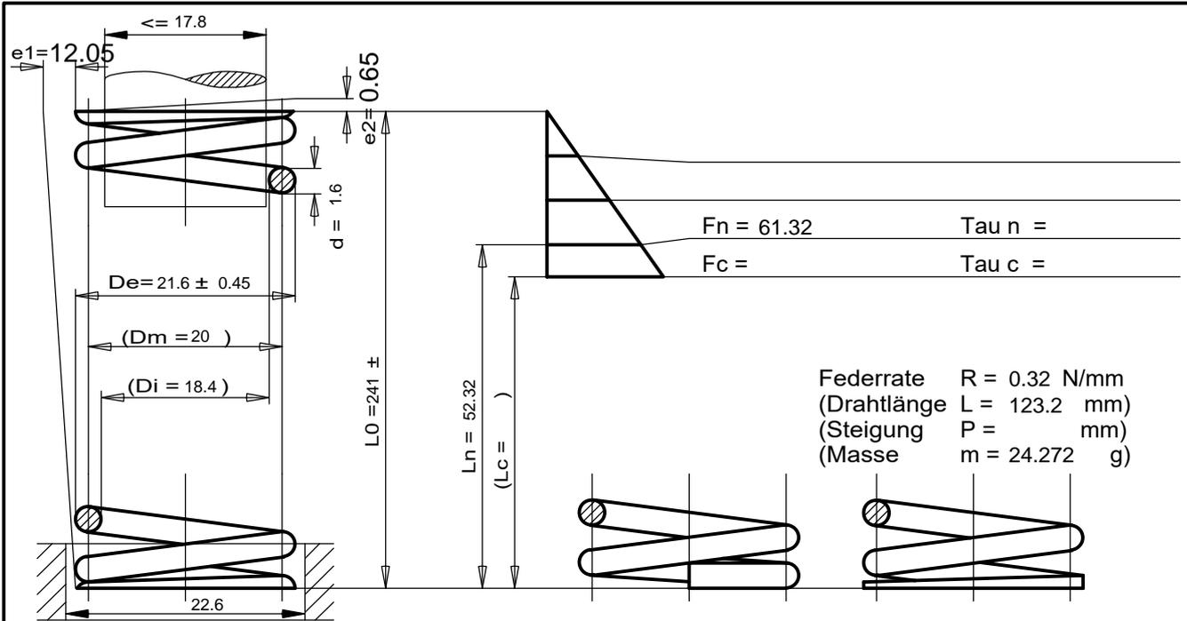
Federrate  $R = 0.32 \text{ N/mm}$
