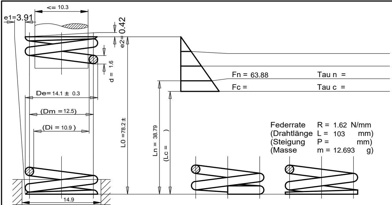
Federrate  $R = 1.62 \text{ N/mm}$
