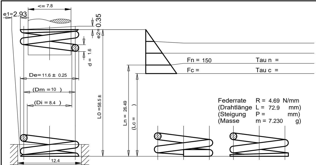
Federrate R = 4.69 N/mm
