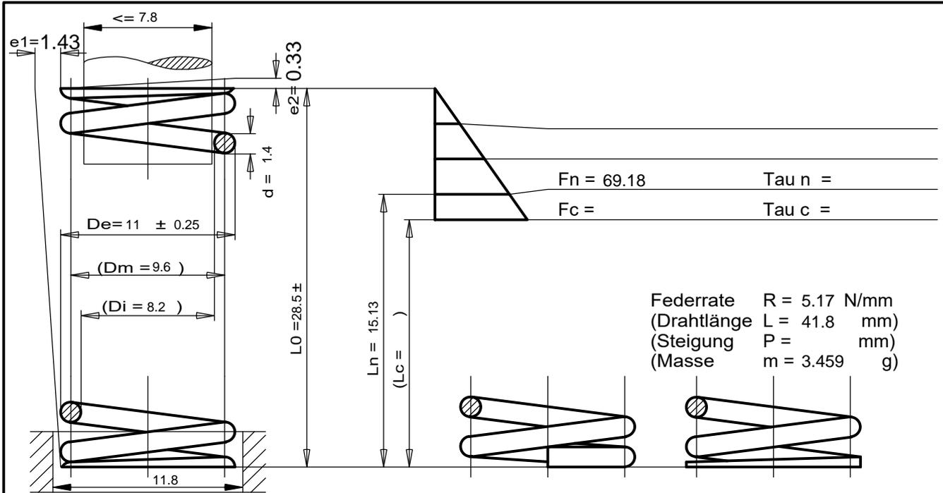
Federrate  $R = 5.17 \text{ N/mm}$
