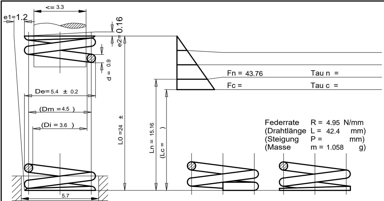
Federrate  $R = 4.95 \text{ N/mm}$
