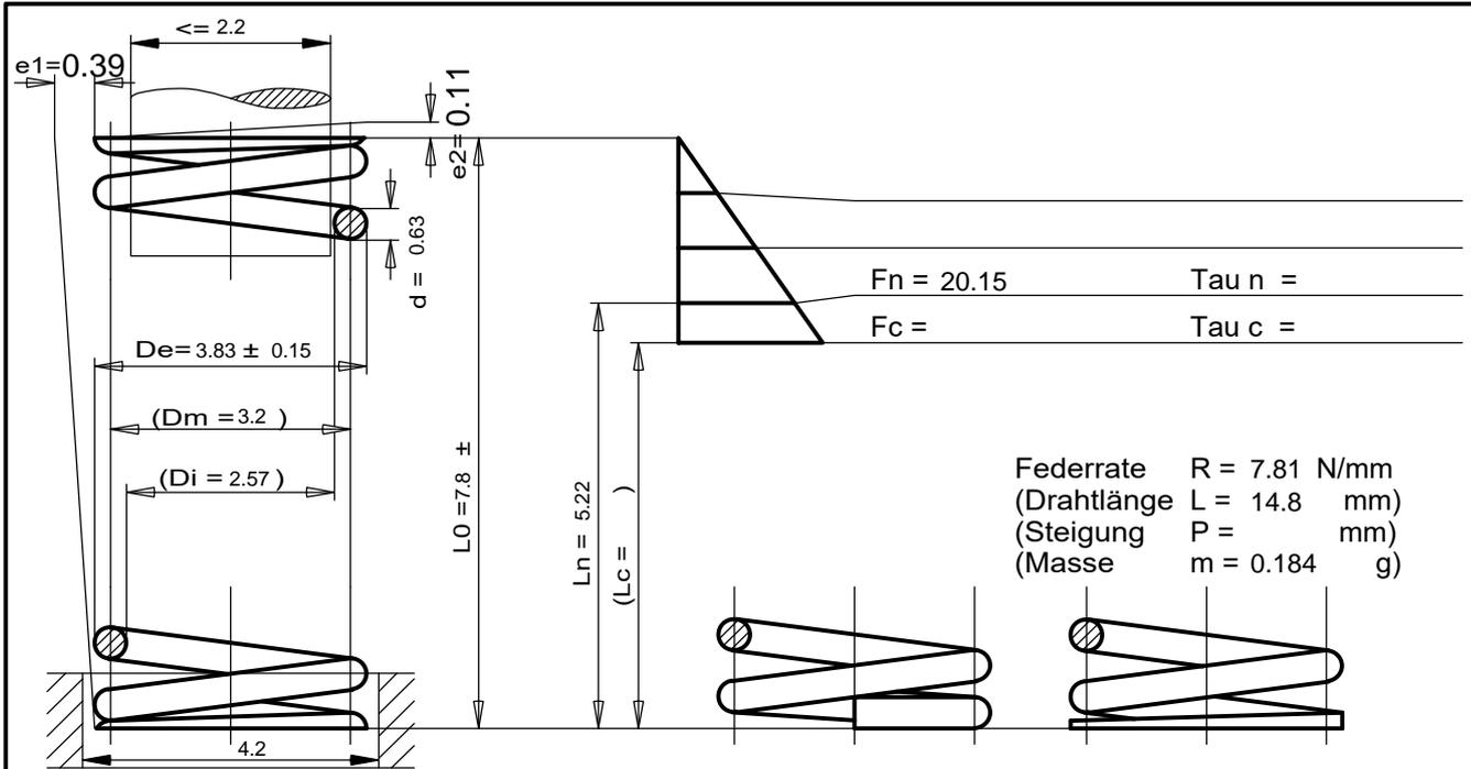
Federrate  $R = 7.81 \text{ N/mm}$
