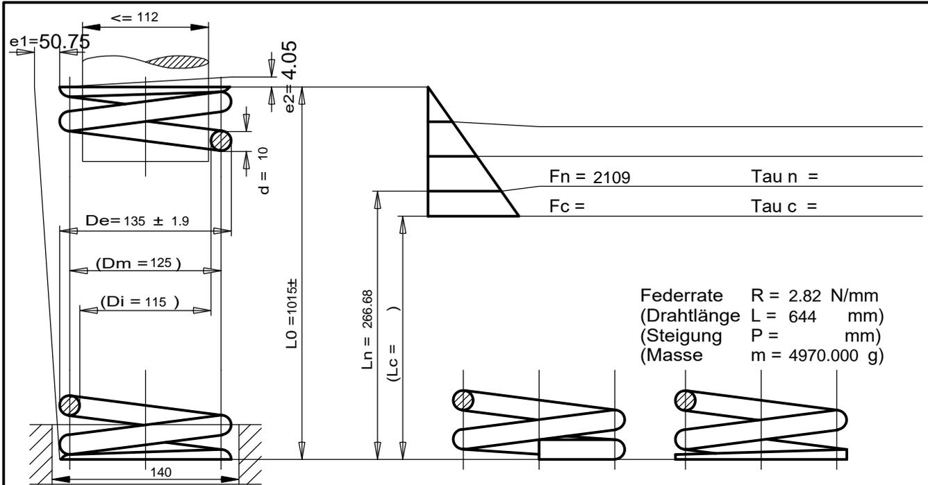
Federrate  $R = 2.82 \text{ N/mm}$
