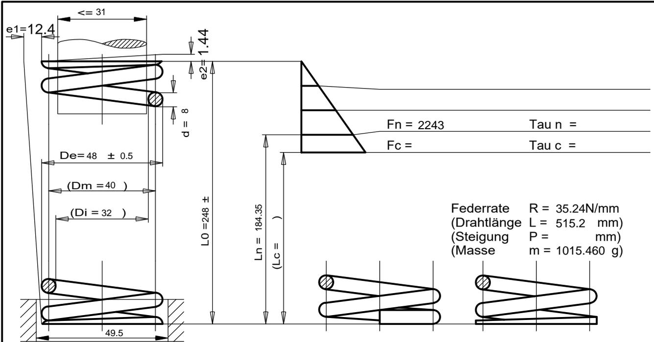
Federrate  $R = 35.24 \text{ N/mm}$
