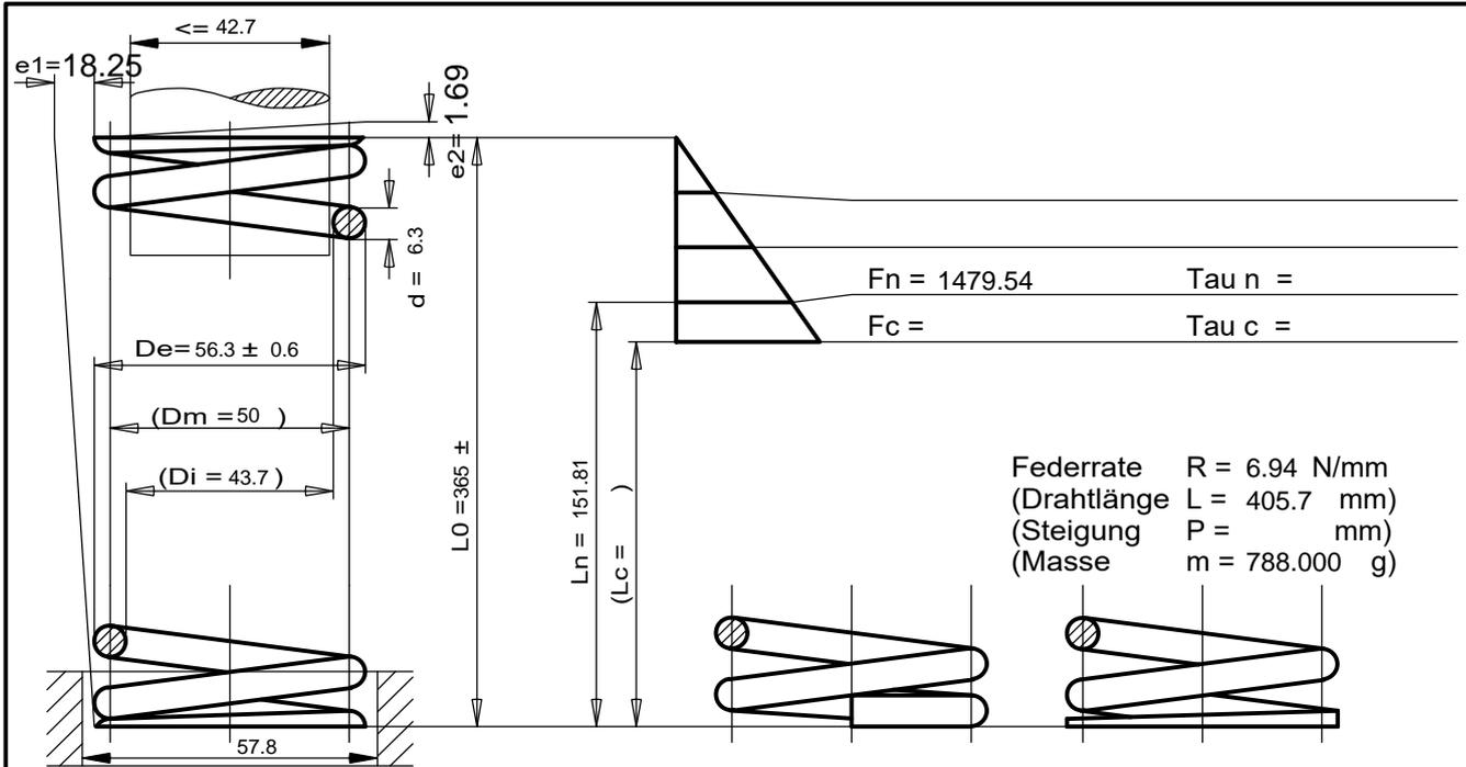
Federrate  $R = 6.94 \text{ N/mm}$
