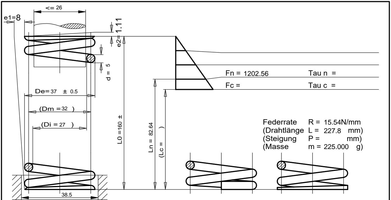
Federrate  $R = 15.54 \text{ N/mm}$
