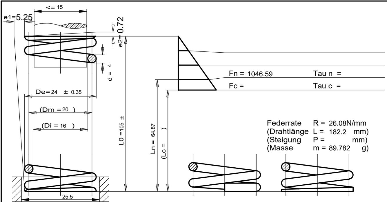
Federrate  $R = 26.08 \text{ N/mm}$
