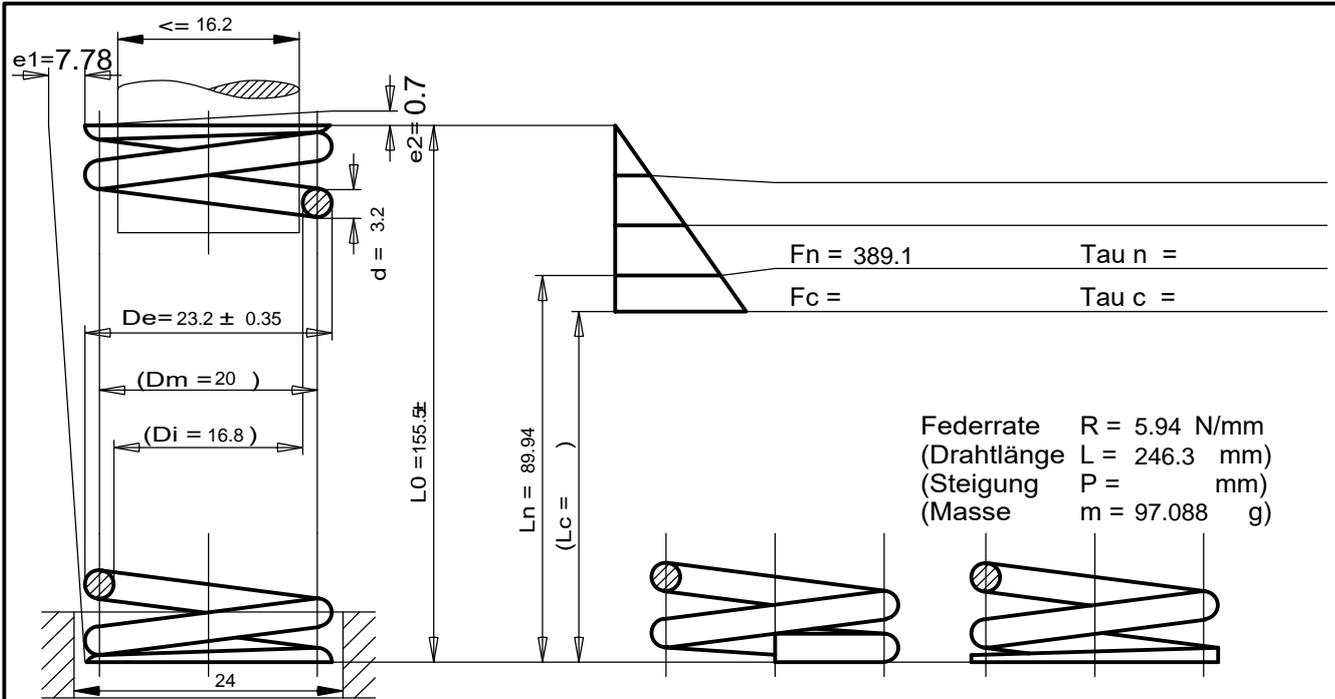
Federrate  $R = 5.94 \text{ N/mm}$
