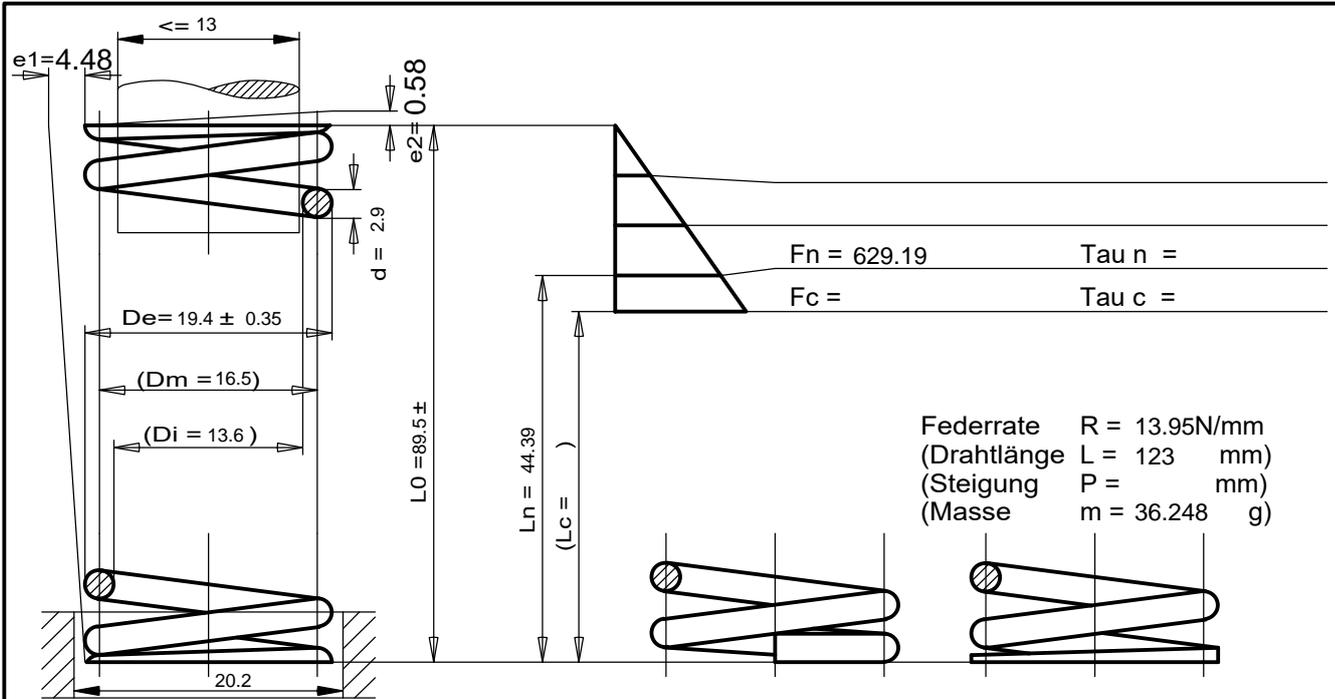
Federrate  $R = 13.95\text{N/mm}$
