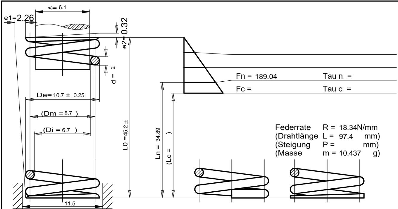
Federrate  $R = 18.34 \text{ N/mm}$
