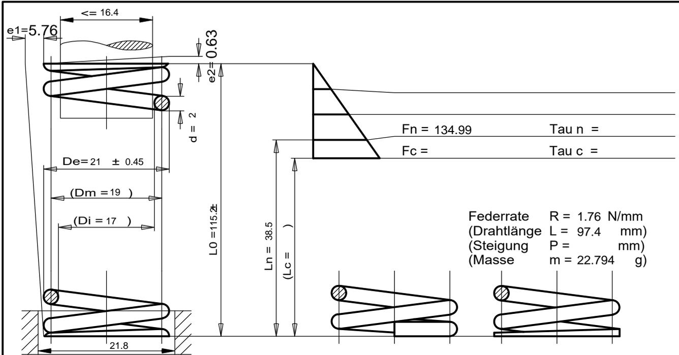
Federrate  $R = 1.76 \text{ N/mm}$
