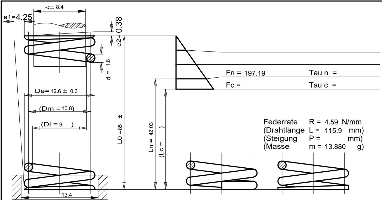
Federrate  $R = 4.59 \text{ N/mm}$
