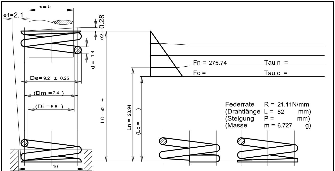
Federrate  $R = 21.11 \text{ N/mm}$
