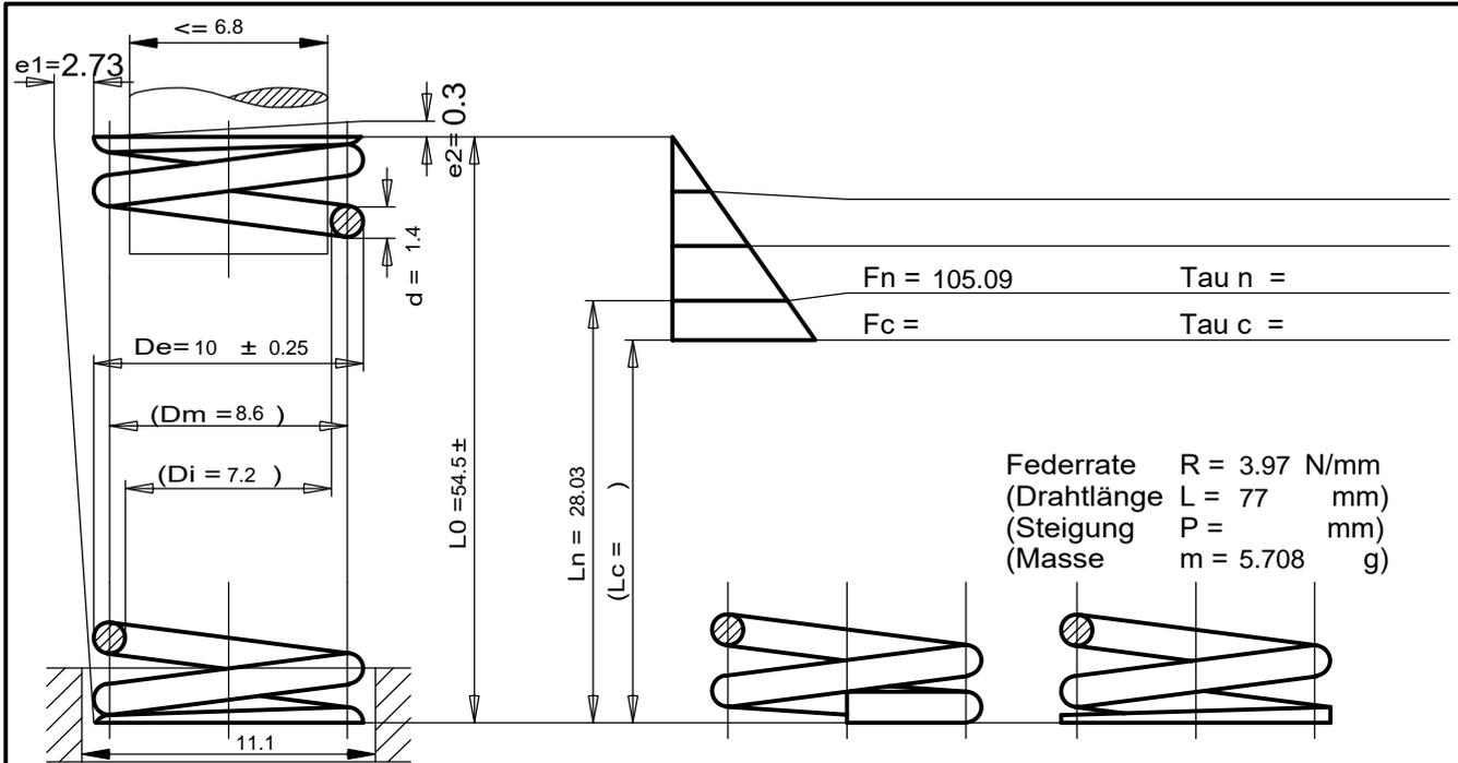
Federrate  $R = 3.97 \text{ N/mm}$
