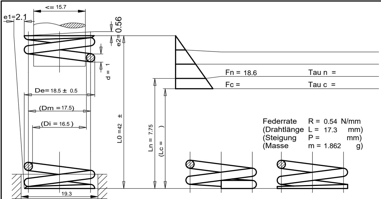
Federrate  $R = 0.54 \text{ N/mm}$
