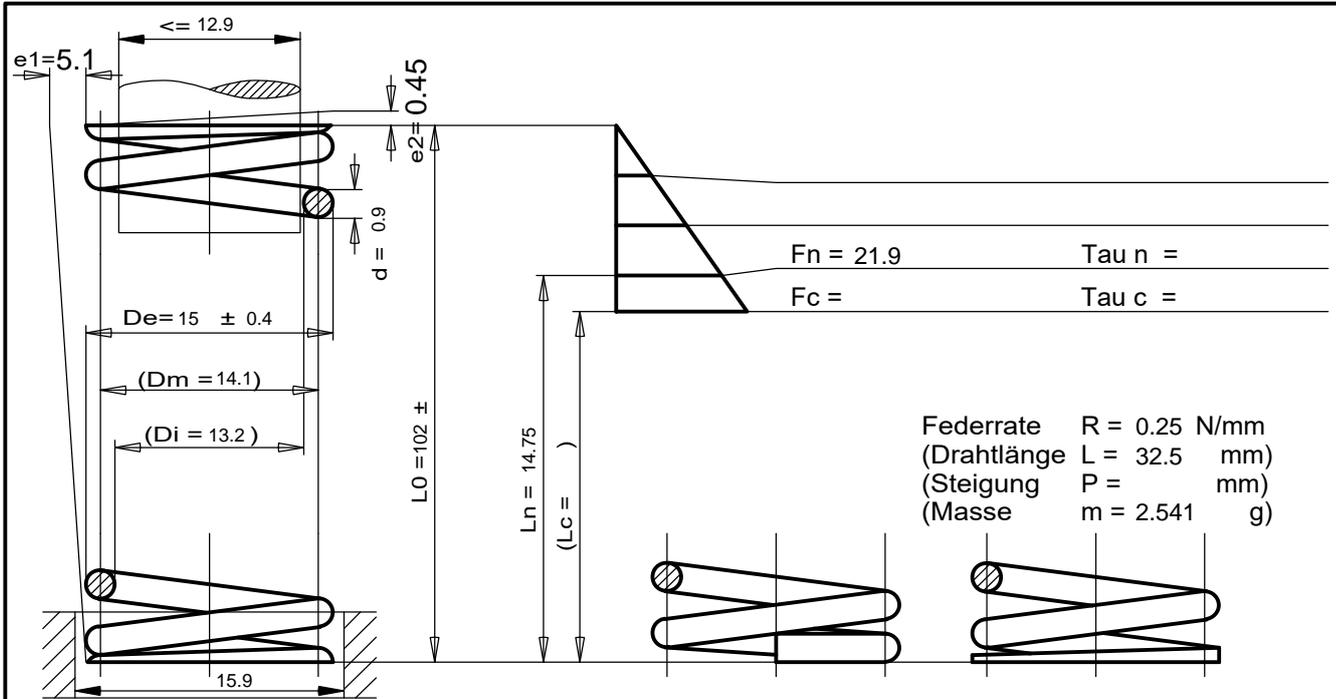
Federrate  $R = 0.25 \text{ N/mm}$
