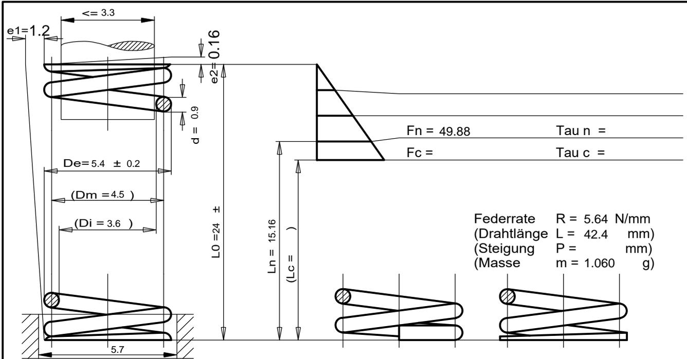
Federrate R = 5.64 N/mm
