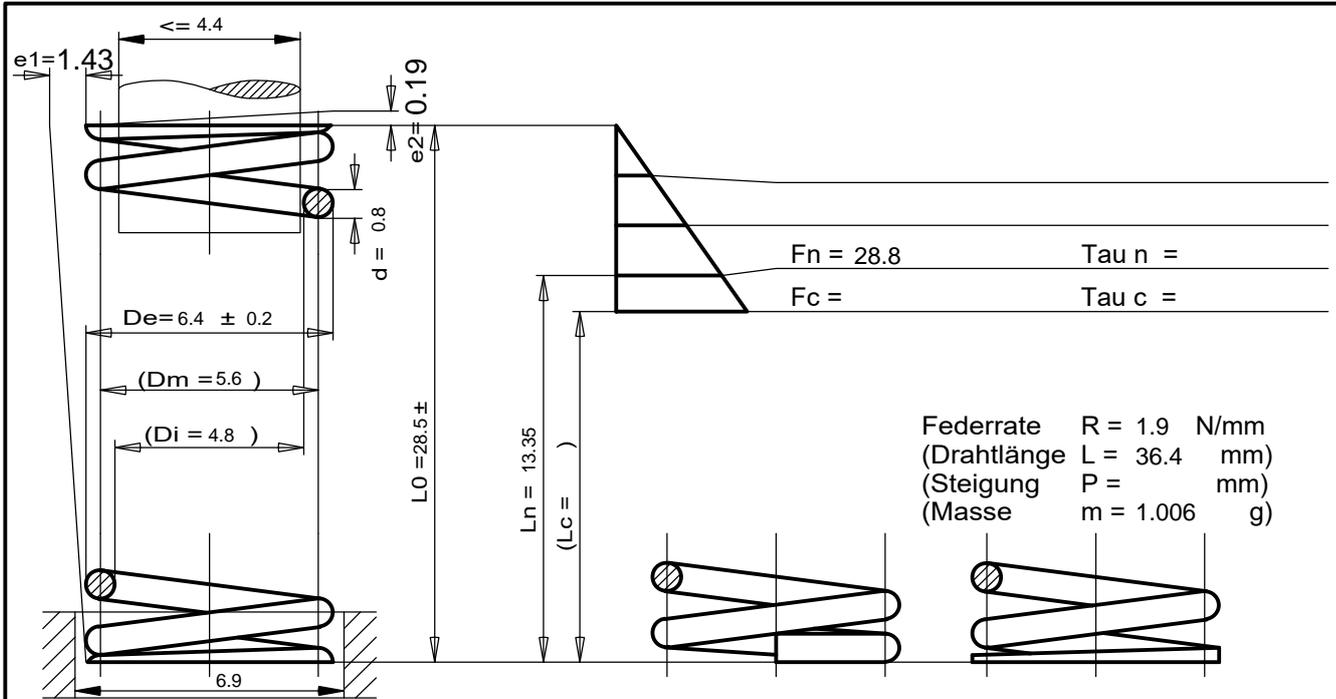
Federrate  $R = 1.9 \text{ N/mm}$
