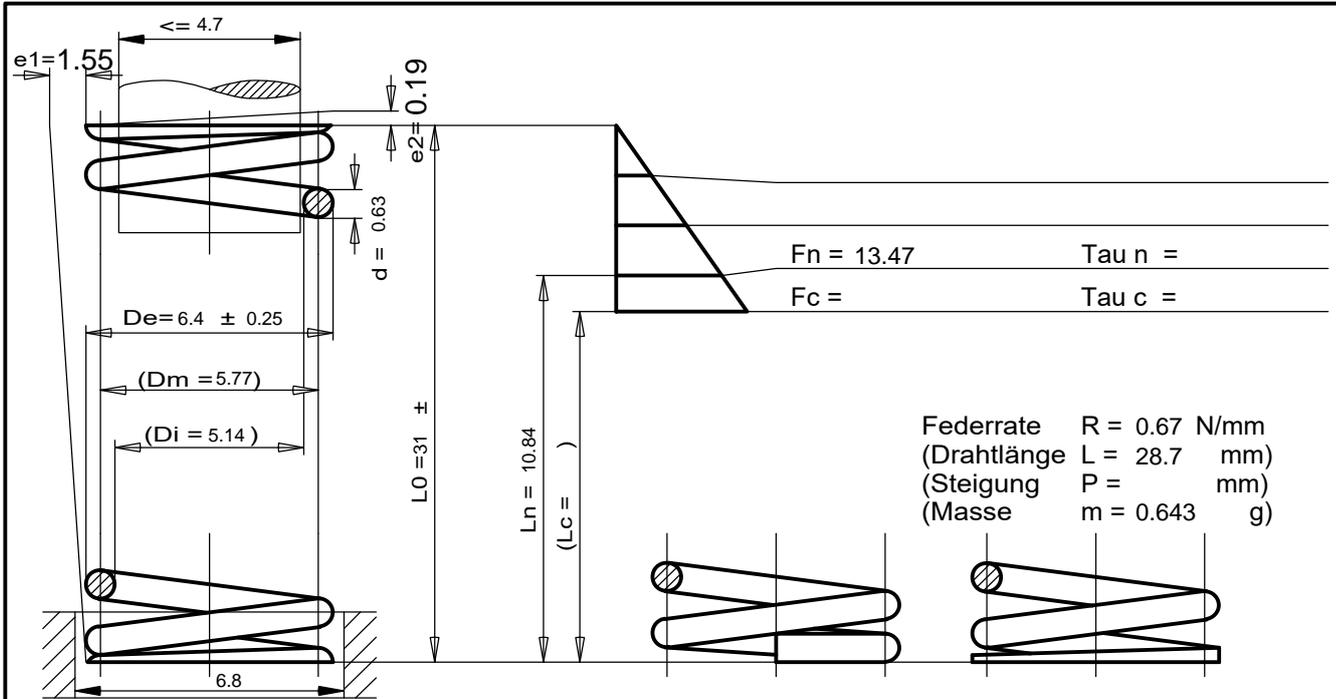
Federrate  $R = 0.67 \text{ N/mm}$
