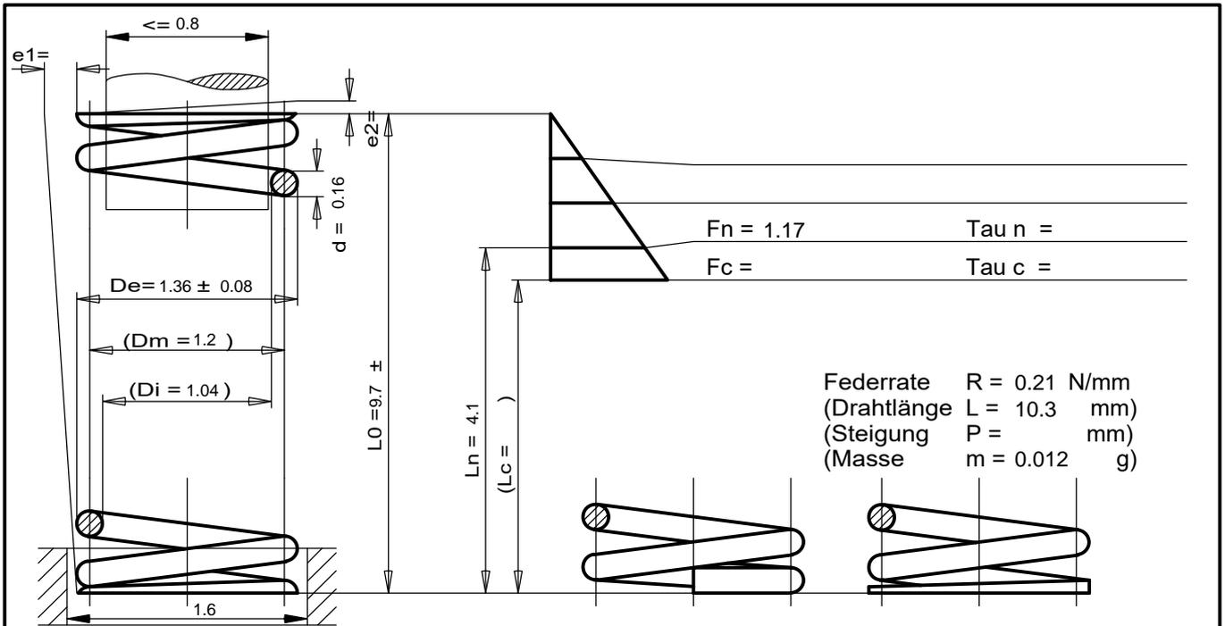
Federrate  $R = 0.21 \text{ N/mm}$
