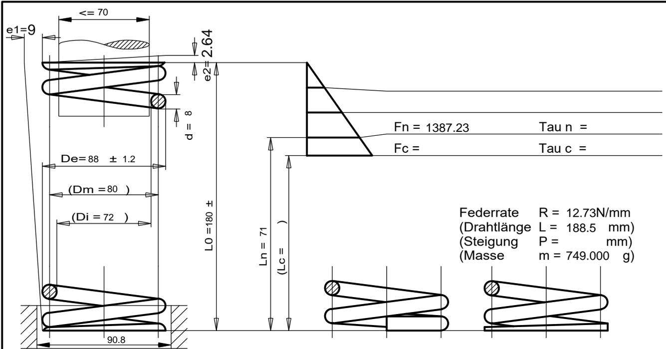
Federrate  $R = 12.73 \text{ N/mm}$
