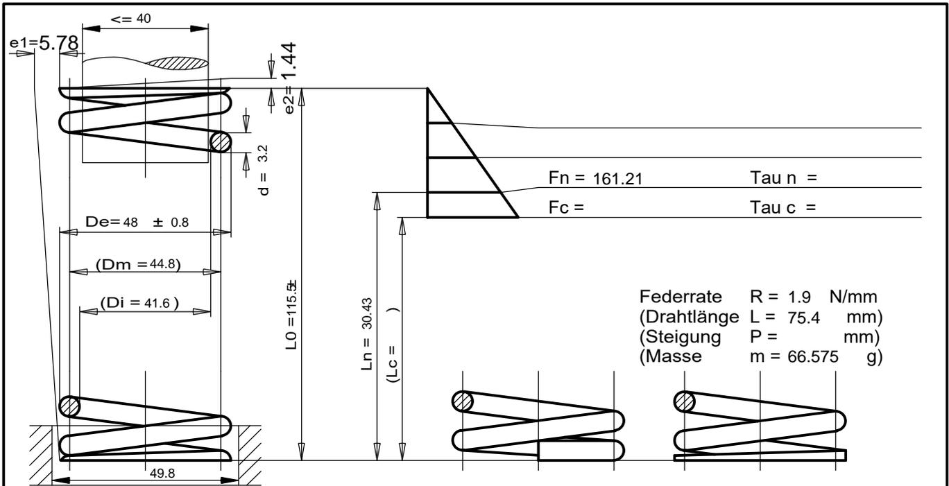
Federrate  $R = 1.9 \text{ N/mm}$
